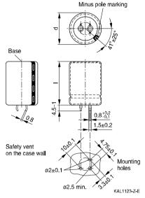
Snap-in capacitors are also available with 3 terminals (length 4.5-1 mm). For packing mode and ordering example see next page.
