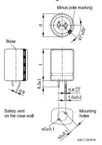
Snap-in terminals, length  $6.3\pm1$  mm. Also available in a shorter version with a length of 4.5-1 mm. For packing mode and ordering example see next page.
